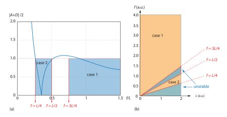
Figure SB.10 Stability condition and areas for a resonator with length L and in the prescence of a thermal lens with focal length f.
