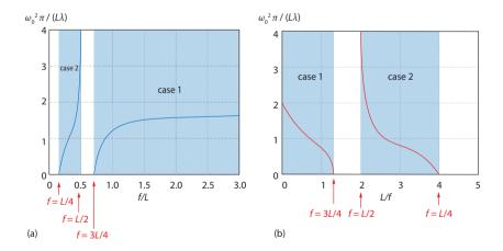
Figure SB.11 Waist radius at output coupler as a function of (a) the focal length and (b) the refractive power of the thermal lens.
