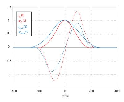
Figure SB.12 Pulse envelope and frequency chirp in a Gaussian and a  ${\rm sech}^2$  pulse in a nonlinear medium.
