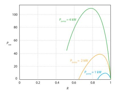
Figure SB.4: Output cw power for various pump powers as a function of the outcoupler reflectance.
