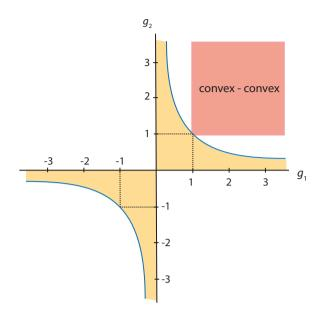
Figure SB.8 Stability diagram for convex-convex laser resonators.
