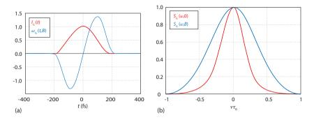
Figure SB.13 (a) Pulse envelope, frequency spectrum, and (b) power spectrum of a Gaussian pulse after passage through a nonlinear medium.
