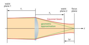
Figure SB.2 Gauss beam transformation through a telescope systems.
