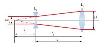
Figure SB.1 Ray diagram of a Galilei telescope.
